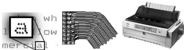
Figure 2.15: Dot Matrix Pins
